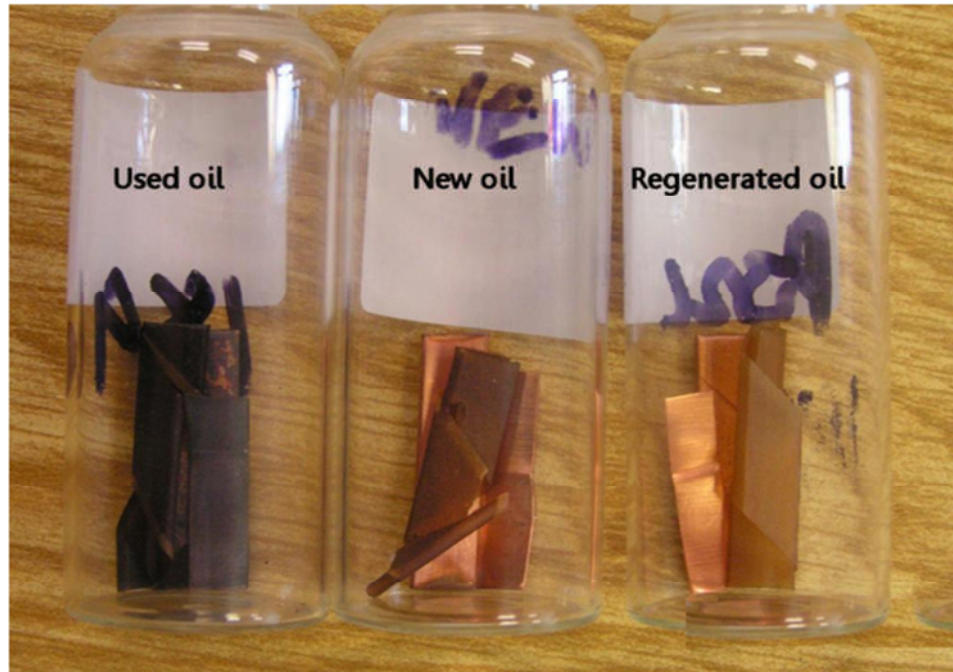
Above: Corrosive sulfur tests on used, new and regenerated oils per ASTM 1275 Method B
