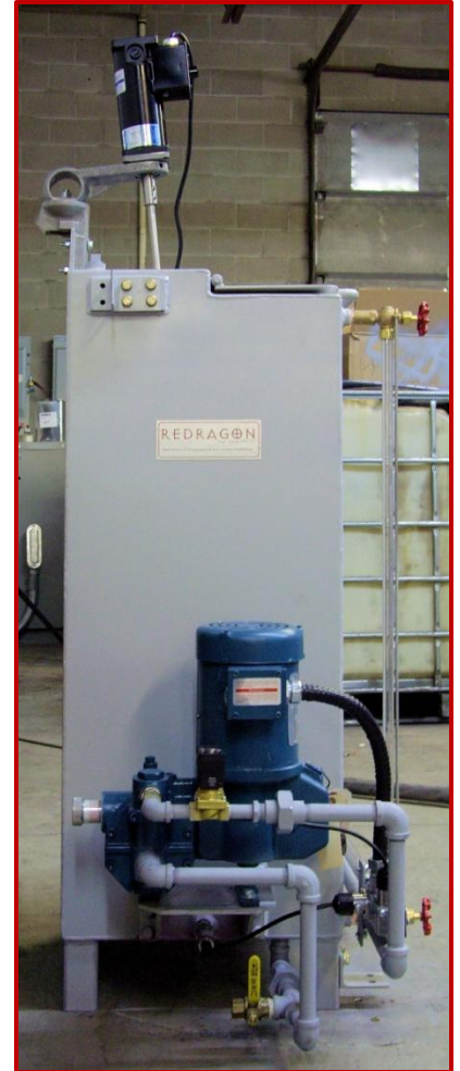
(above) The Series DBPC Anti-Oxidant Inhibitor System can be retro-fitted to any degasifier.
